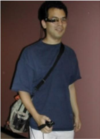
An example wearable computer usage pattern with head mounted display and one handed keyboard.
