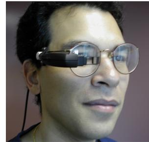
Figure 1: Wearable Computer Headmounted Display
