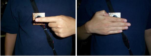
Figure 6: Moving the left index finger up and down causes zooming. An open palm stops movement.
