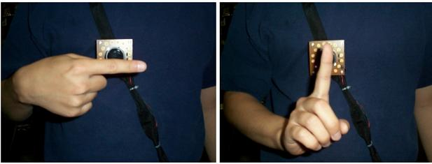
Figure 5: Moving the right index finger up and down causes vertical panning. Moving a vertical index finger left and right causes horizontal panning.
