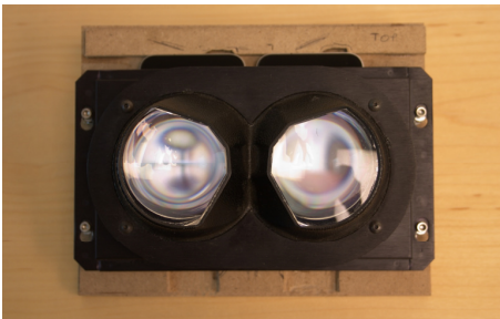
Head mounted display with a LEEP-type lens assembly in place.
